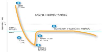
Advanced osmometers utilize the industry-preferred freezing point depression method to determine the osmolality of an aqueous-based solution. When a solute (particles) is dissolved in a solvent (water), the freezing point of that solution is lowered compared to that of the solvent alone. As more solute is added, the freezing point decreases further. Therefore, by precisely measuring the freezing point of the solution, the osmolality (i.e., concentration) can be determined.
