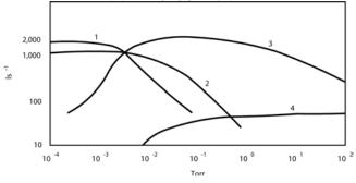
In their most efficient range, booster pumps (1) fill the gap between the pumping speeds of vapor diffusion pumps (2), vapor booster pumps (3) and rotary or dry high vacuum pumps (4).
