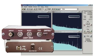
EASY-MCA interfaces to a PC via a USB2 cable. This compact MCA is stackable and portable, and no PC option slots are needed. Each EASY-MCA has memory capable of holding the complete spectrum. You have the option of 2k channels of resolution which can be switched to 1k or 0.5k channels or 8k channels of resolution which can be switched to 4k, 2k, 1k, or 0.5k channels.
