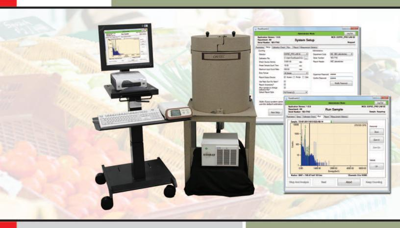
High Resolution Germanium Gamma Spectroscopy Workstation for Quantitative Determination of Radionuclides in Food
