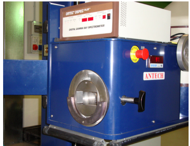
Close up of the detector with the optional interchangeable collimator
