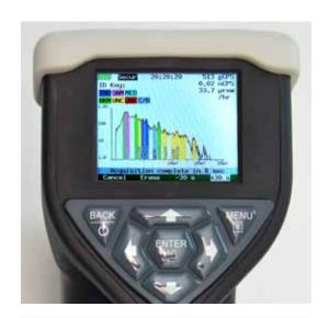
▲ The RIIDEye X operator can view the real-time spectra build of isotopes present in the environment as the identification scan is in process.
